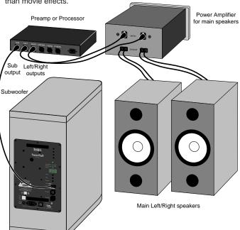
If your main speakers play sufficiently loudly for all your uses but do not reproduce the full low frequency range of the left/right channels, you should also use the subwoofer to augment the bass response of your main speakers. This can be accomplished without altering the signal or wiring to your main speakers by using one of the next two configurations.
